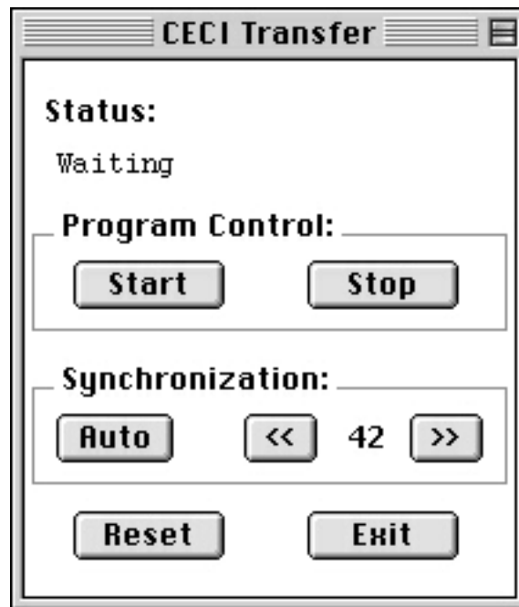
Figure 3.7: The download window. The window includes a status area at the top and buttons to start and stop the program currently on the CECI. The bottom half of the window includes controls to manually manage the communication process, which is insufficiently robust to handle the adjustments automatically.
