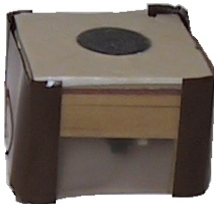
Figure 2.4: The smart tile prototype. The base is three inches square and stands two inches tall. The tile is made from a polymer clay with a tinted plastic window set in the center. The electronics, communication, and power connections are mounted in the base under the tile.
