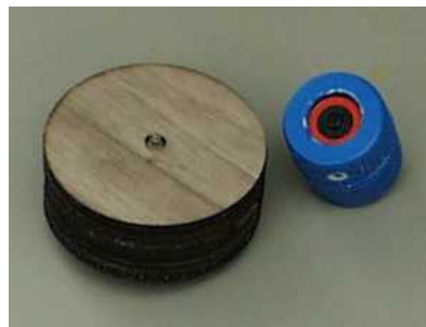
Figure 2.5: Two versions of the Rototack. The figure on the left is the final version (Mark III) and the version on the right is the original version of the Rototack (Mark I). The Mark III's size allows for larger batteries.
