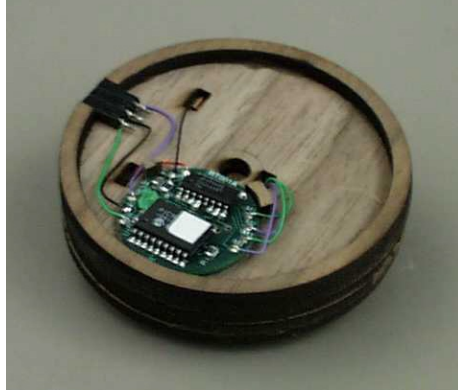
Figure 2.6: A Rototack with the bottom removed, exposing the electronics. The small circular circuit board contains the microprocessor and stepper motor driver.
